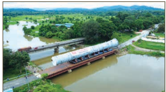
C3 Splitter Column (bottom portion) crossing Kalyani bridge
