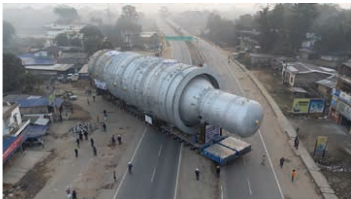
Transportation of VDU Column from NRL Jetty to NREP Site
